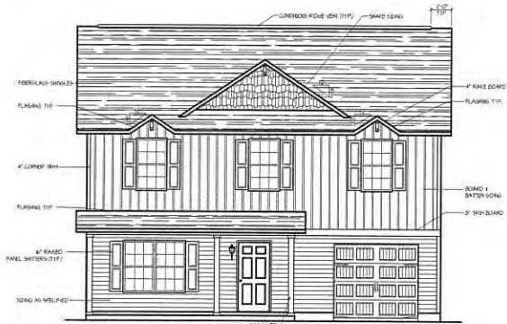
FRONT ELEVATION A 8:12 PITCH NEAR ROOF PITCH = 22-5 1/8"
